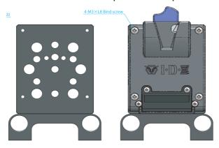
On larger cameras fitted with a V-mount plate, it is possible to fit the A-Vmicro2 plate. It enables two Imicro batteries to be mounted which are discharged sequentially giving a hot swap capability which allows for continuous filming. This A-Vmicro2 fits to all IDX chargers effectively doubling the quantity of batteries that can be left to charge i.e. four Imicro batteries can be charged on a two channel IDX charger.
