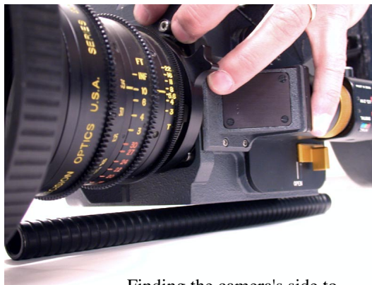
Finding the camera's side to side center of gravity.
