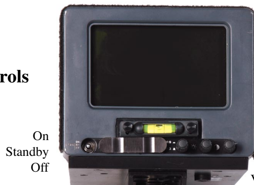
Image flip and invert (slide cover when off to reveal switches)
