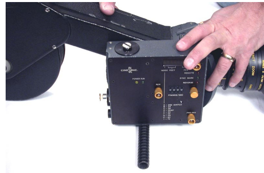
Finding the camera's fore-aft center of gravity.
