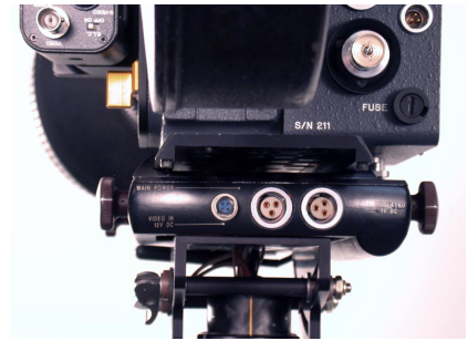
Camera c.g. centered over post – side to side.
