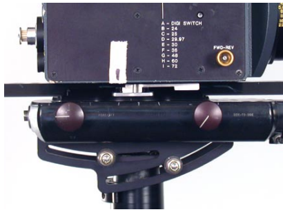
Camera c.g. .75" behind center post – fore-aft.
