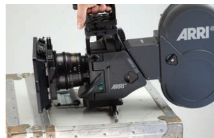
Finding the camera's fore-aft center of gravity.
