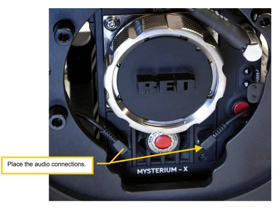
Plug in the optional Submersible Mic, Hydrophone, or Comm input to Mic-1 or Mic-2 locations on the EPIC / Scarlet cameras
