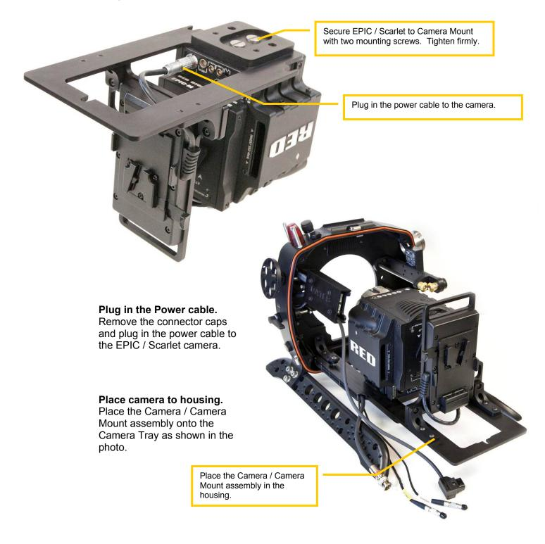
**Connect External LCD.** Slide the assembly forward until 2 in / 5 cm from fully seating into the housing. This is a good point to connect the LCD cable on the front of the EPIC / Scarlet camera.
