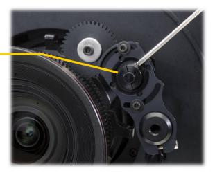
**Set the focus/iris indicators.** The left side Focus control and right side Iris control have focus and iris dials. These shipped in the parts kit. These may be aluminum and pre-marked for the lens, or white plastic for marking focus / iris indications yourself.
