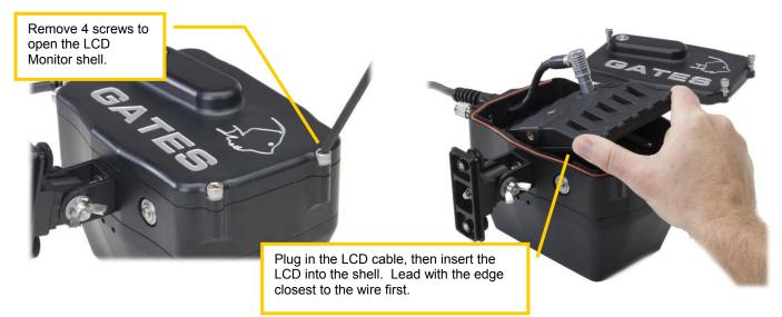
**Clean the window / LCD.** If necessary, clean the inside of the window and blow out any foreign matter. Clean the LCD screen as well.
