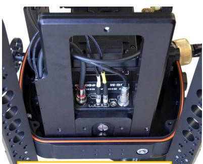
Tilt the housing forward and plug in the SYNC and CTRL Connections. The connectors are clearly marked.
