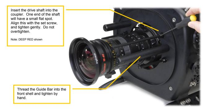
**LGD's mounting.** Install the LGD's in their proper orientation with pivot gear screws facing forward. Slide it onto the guide bar and drive shaft, then line up the LGD with the lens gear you wish it to access.
