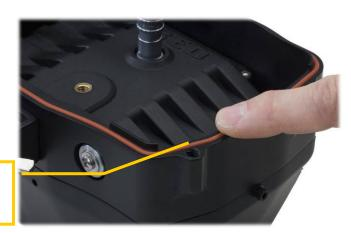
Inspect the o-ring. Wipe clean with your finger to remove foreign material. DO NOT lubricate orange o-rings.
