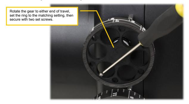
**Verify Operation.** Once positioned and secured check operation of the Focus and Iris controls. They should rotate freely – but with slight resistance – in both directions and through the entire range of travel. If not, repeat steps 1-3.
