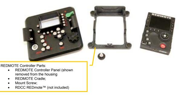
**Install REDmote<sup>TM</sup>.** Insert the REDmote<sup>TM</sup> at an angle as shown in the photo. It will fully seat into the cradle. Secure with the small thumbscrew.
