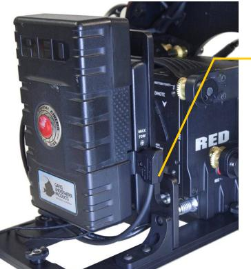
Install the Power connector here, on the side of the V-Lock battery mount.
