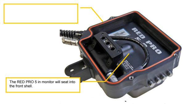
**Close the monitor shell.** Mate the rear shell to the housing. Insert and tighten the 3 screws until snug. Tighten until there is no visible gap between shells. A good indicator is when the orange o-ring is no longer visible.
