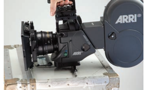
Finding the camera's fore-aft center of gravity.
