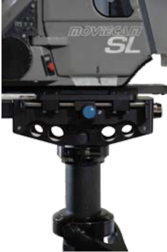
Camera's fore-aft c.g. .75" behind center post.
