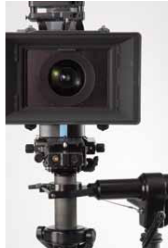
Camera c.g. centered over post – side to side.
