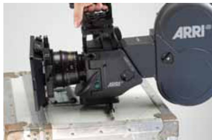
Finding the camera's fore-aft center of gravity.
