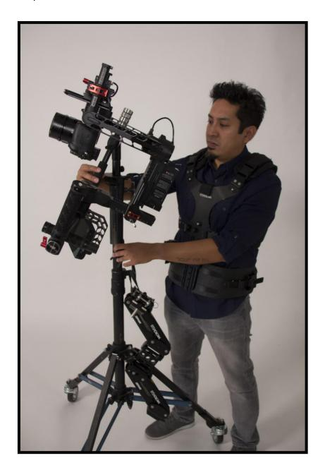
If the tilt behavior is heavy, that means your system is **too** bottom heavy. But instead of removing the weights, which you can use later for fine-tuning, we'll move the Post Block down the Post.
