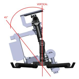
If the Steadimate is between 45° and horizontal, confirm that the Post Clamp is set at number 0 and try adding 2 more Balance Weights. You may also remove or change your accessories to lighten the system.
