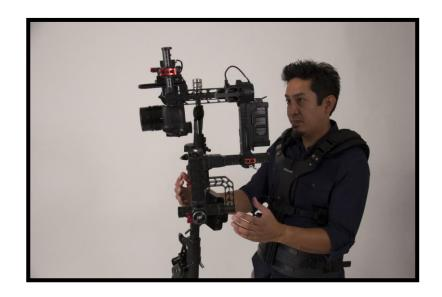
If necessary, go back and re-center the Steadimate using the Tilt Balance Knob as previously described on page 4-2 of this manual.
