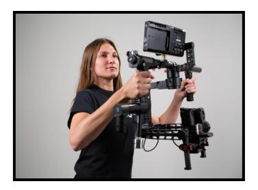
Before we explore Steadimate Operating, remember that you're still able to pick up the motorized gimbal by hand for traditional operating. No need to replace the original hand grip or rebalance the Steadimate.
