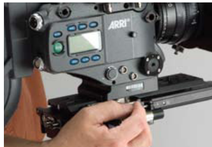
Closing the locking lever.
