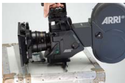
Finding the camera's fore-aft center of gravity.
