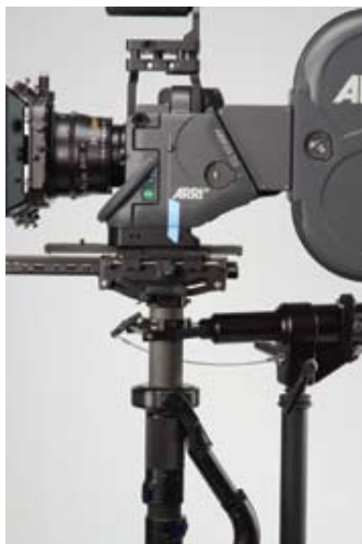
Camera c.g. .75" (19mm) behind center post – fore-aft.
