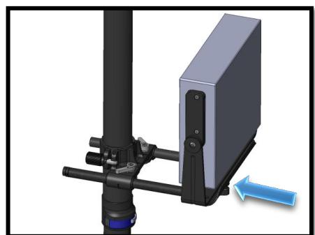
Test the holding power of the rod clamps to ensure the monitor or batteries will not slide when locked.
