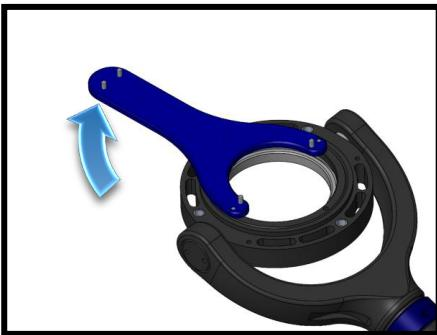
Install the pan bearing lock. Hand turn first to ensure proper threading, then finish with the "outer" pins of the spanner.
