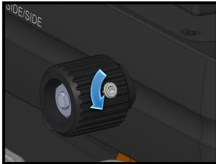
Loosen the locking set screws one-half turn with a 1/16" Allen wrench. You do not need to remove the set screw.
