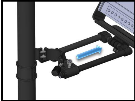
Pull the monitor away from the post. The post clamp will swing clear, leaving the brake on the post.
