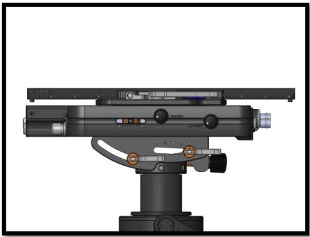
To remove the stage from the post, start with the tilt set square, which allows access to all screws.
