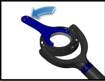
Use the "outer" spanner pins to unscrew and remove the pan bearing lock.
