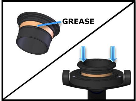
If necessary, lightly grease the inner ring and install with even pressure. Use as little grease as possible to install. Attach the top cover.
