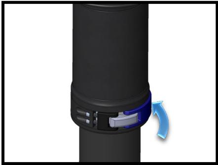
The over-center locks on the post clamps are adjusted while the post clamp is closed.
