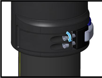
Use a 3/32" Allen wrench to turn each screw an equal, tiny amount. You don't want to over-tighten these, take your time.
