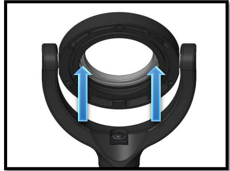
Applying even pressure to both sides, ease the pan bearing out. Never use tools to pry on a bearing.
