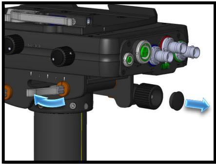
With no camera on the rig, open the cam levers and remove the cover from the tilt drive knob with a penknife or thin screwdriver.
