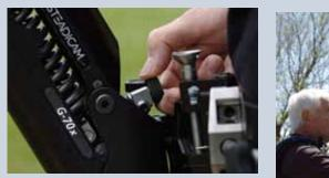
Adjusting the ride: the arm must be angled up at the top of its range. Note: the ride knob is horizontal, the lift knob is vertical.
