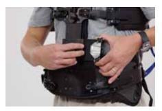
On the arm, pull the "parachute pin," flip the mating block, and reinsert the parachute pin with the kick back link rotated (see page 6). Note that the mating block is now reversed; the upper side to side adjusting screw is now the lower screw and vice versa.
