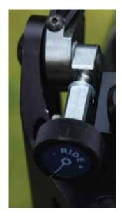
Start by presetting the Ride knob to the middle of its travel (about 20 threads visible). Once you get the iso-elastic feel you like, make a note of the threads and the camera weight for future reference.
