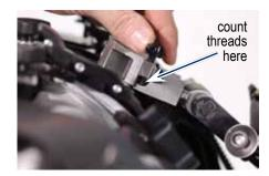
The "in-out" adjustment on the socket block varies greatly by the operator's body type. If you have big pectorals and a flat stomach, the top screw is almost all the way in. If you've been eating well and exercising less, the top screw will be further out.
