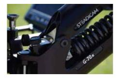
When the forearm section is set correctly, adjust the upper arm section to follow (track with) the upper arm section as you boom fully up and down. Do not worry if the arm tends to lock up or down at this point. Note that the Lift knob has a range of adjustment of 32 turns. This means that each turn of the Lift knob will add or subtract about 1.5 lbs (.68kg) of lift.
