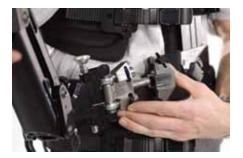
The G-70x<sup>™</sup> arm socket is inserted into the socket block on the vest.
