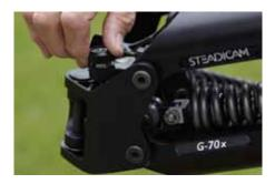
Slightly raise or lower the arm segment to find the sweet spot. Adjust the arm's lifting power so that the arm section seeks a position slightly above horizontal.
