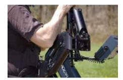
Lift can be altered by forcefully holding the arm segments at the correct angle while adjusting, but be prepared for some exertion! You might be shocked how energetic the springs feel if you are raising or lowering the lift by 30 lbs (14kg)!
