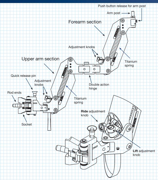
The G-50x is the second release of Tiffen's G-Series arms. The revolutionary, patented Geo spring geometry optimizes performance throughout its lifting range. It tames high/low arm travel with adjustable-length crankshafts that dynamically rock the spring termination as the arm is boomed up or down. Powered by titanium springs, the G-50x arm smoothly carries any load from 12 to 50 pounds (5.4 to 23 kgs). The all new bearing performance enhancements on the G-50x arm
