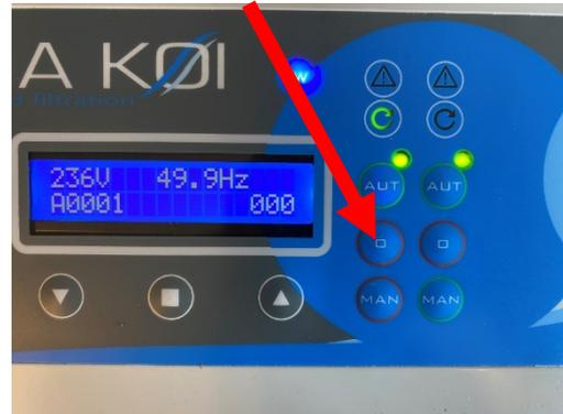
**THE GREEN LIGHTS MUST BE ON AT ALL TIMES! OTHERWISE, THE SYSTEM IS OFF OR WILL NOT BE RINSED! MAKE SURE YOU CHECK THIS**
