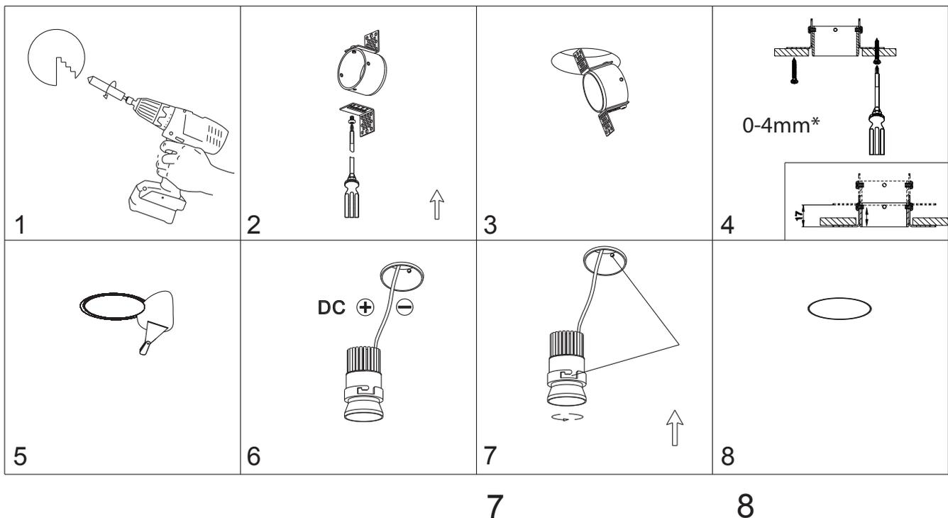
\* When plastering the ceiling after installation mount frame 2-4 mm out of the ceiling. This depends on the plaster thickness. Please discuss with your plasterer. For example, when plaster will be 3mm thick, the trimless frame should stick out 3mm. After plaster it will be 0mm (frame / ceiling will be flat surface.)
