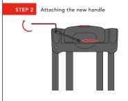
Insert a 0.5" screw into the top of the handle and hand tighten the 8mm lock nut to the bolt. Use the 8mm combination wrench to firmly hold the lock nut. With your other hand, insert the 3mm Allen wrench into the bolt head and turn clockwise to tighten. Repeat on other side.
