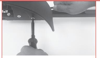
4. Attach the left fender using a 35mm bolt and the nut from Step 3. Pass the bolt through the top hole in the fender from the outside, through the square tube into the nut. Do not fully tighten.
