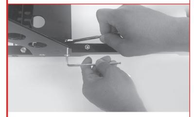
3. Remove the top bolt that attaches the side panel to the square tube. You will not need this bolt, but set aside the nut for Step 4.
