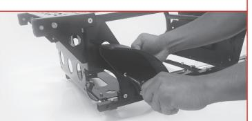
6. Line up the lower hole in the fender with the nut inside of the fender lock. Use a 16mm bolt to secure. Tighten fully and then tighten the bolt from Step 4.
