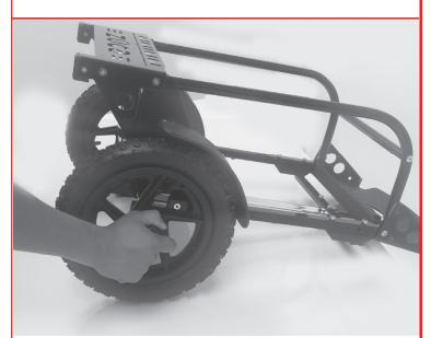
Reinstall the wheels, spacer and axle.
