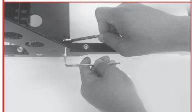
3. Remove the top bolt that attaches the side panel to the square tube. You will not need this bolt, but set aside the nut for Step 4.
