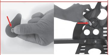
Snap a 10mm nut into a fender lock.
