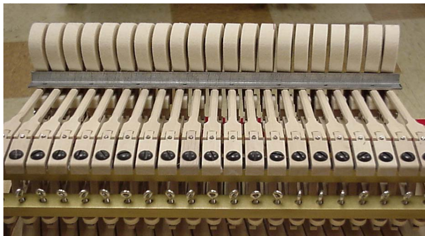
Figure 5 Rail sectional overhang
