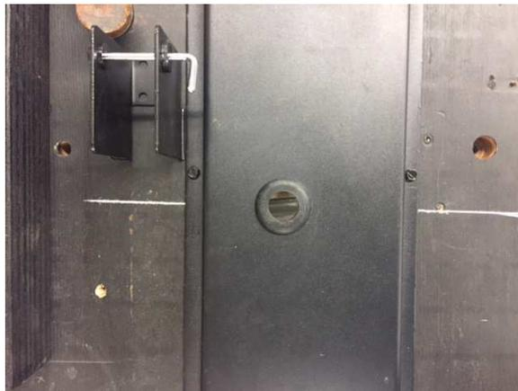
Illustration 87 – Sostenuto hole drilled with grommet in place
