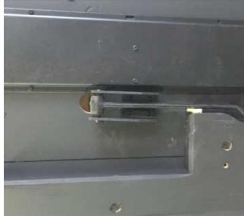
Illustration 14B - Shift Lever Brackets Installed
