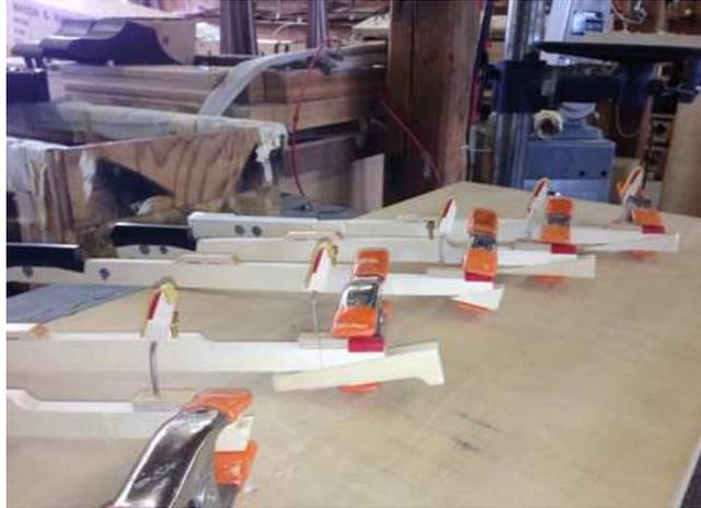
Illustration 10 – Replacing the cut out of the keys
