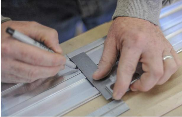
Illustration 57 - Marking cut line on rails
