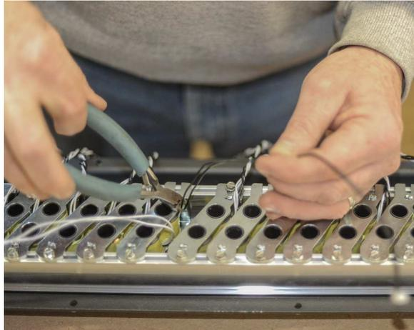
Illustration 123 - Cutting wires on unused solenoids.
