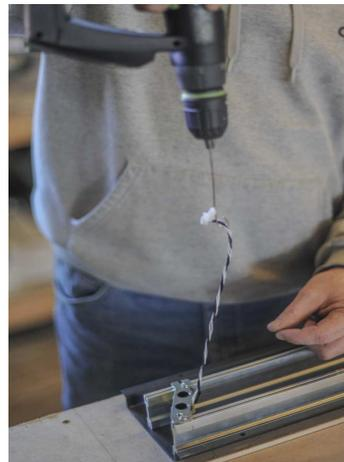
Illustration 125 - Twist solenoid wires
