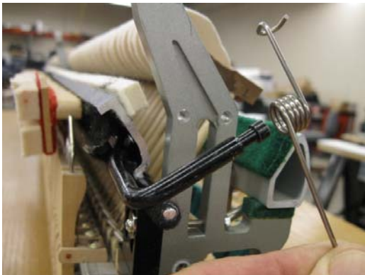
Illustration 28 & 29 – Installing Actuator Return Spring
