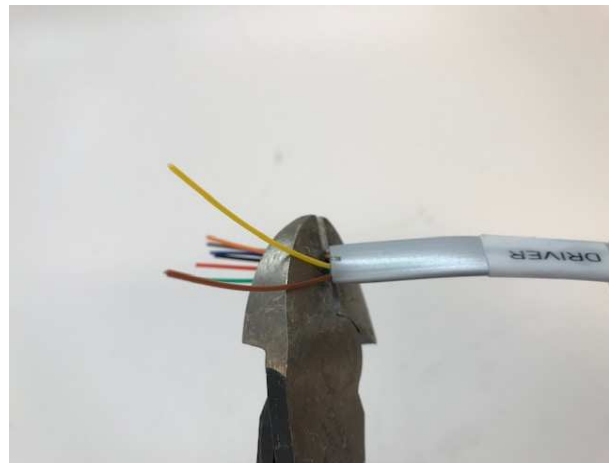
Cutting off unused wires
