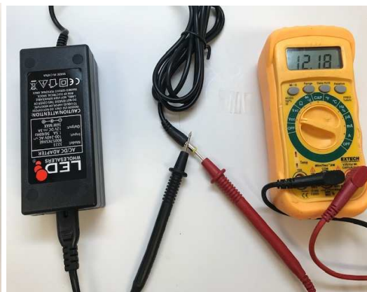
Checking small power supply
