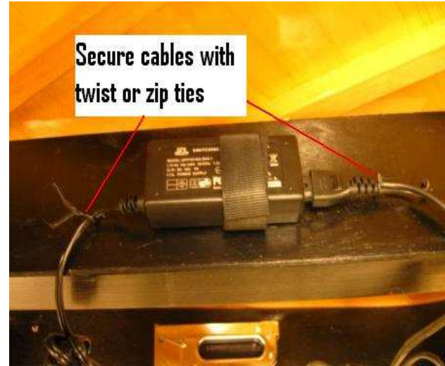
Illustration 138 – 12V power supply on rim
