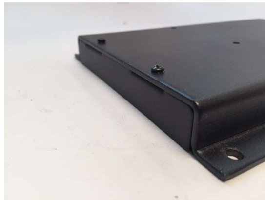
Illustration 63 – End plate installed
