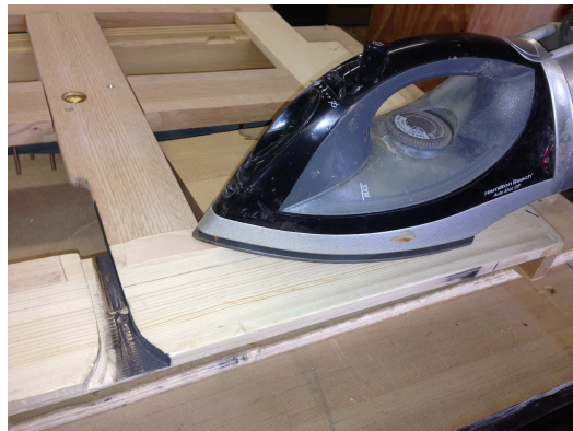
Illustration 29 - Ironing on veneer
