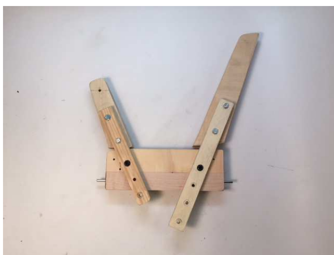
Ill. 90 – Adjustable sostenuto jig (push type)
