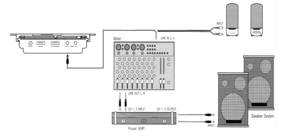
You can also connect an external audio source, such as a CD player, to the QuietTime audio LINE IN port. Connect one end of an audio cable to your audio source's AUX or Line OUT port, and the other end to QuietTime's audio line IN port.
