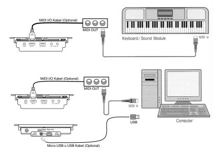
To receive MIDI data from the MIDI keyboard/synthesizer or computer connect the MIDI-OUT cable of the external MIDI device with help of a MIDI cable to the QuietTime's MIDI IN port.
