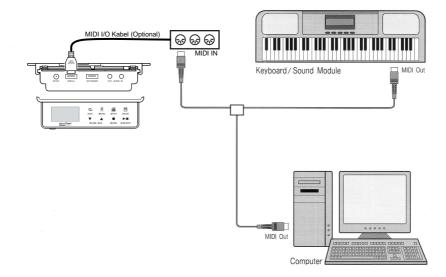
INFO: You can have MIDI IN and OUT cables connected at the same time. If you are using a computer, make sure the "Pass Through" is switched off in your software. This prevents double notes from being played or recorded.
