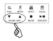
If a key's sensitivity has to be readjusted, use the Up and Down arrows to increase or decrease the volume of the last key that you pressed. This helps you to match the key's sensitivity to that of adjacent keys.
