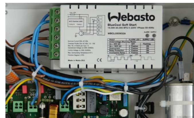
Soft start device available as an option
