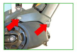
2. On the left, loosen the screw (1) shown on the left with a 6-inch Allen key. The screw remains in place and serves as a hinge for the engine to be folded down (2).
