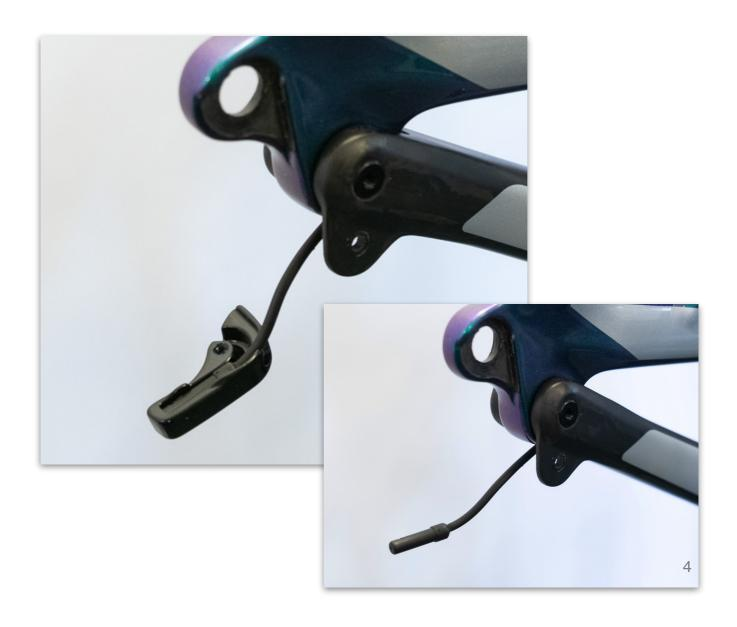
4. Separate the sensor from the bracket.
