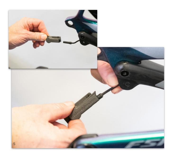
5. Insert the sensor completely into the adapter so that only the cable protrudes and the snap lock is flush with the surface of the adapter.
