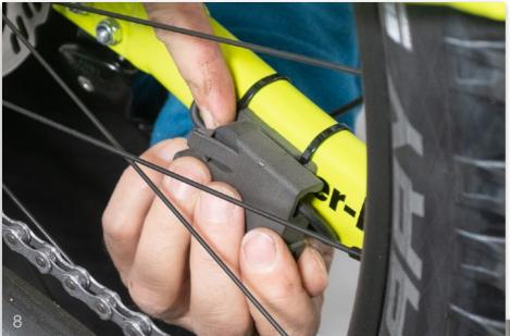
8. Slide the badassBox onto the adapter until it clicks into place.
