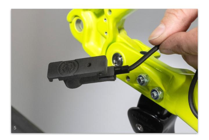
5. Insert the sensor completely into the adapter so that only the cable protrudes and the snap lock is flush with the surface of the adapter.
