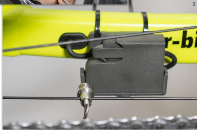
9. Mount the supplied spoke magnet and align it with the edge of the badassBox housing. That's it. Have fun with your faster e-bike!
