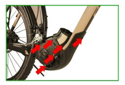
**11.** Loosen and remove the 3 screws of the left engine cover with a suitable Allen key. Then remove the cover.
