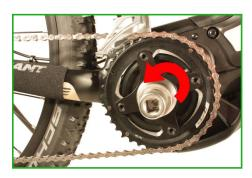
Remove the chain from the chainring and pull out the chainring.
