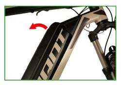
**2.** Loosen the 4 screws of the battery holder with the Allen key.
