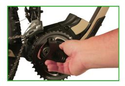
To remove the side panel parts, you must first lift the battery holder gently. The two tabs must be pushed out upward from the side panel parts. Be careful, do not tear off any cables!
