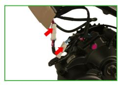
**14.** Connect the 4 connectors of the bikespeed-RS with the corresponding counterparts of the newly disconnected connections.
