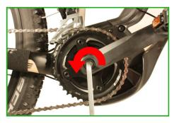
Pull the right crank handle with a suitable crank puller. Screw the puller into the thread of the mounting bolt that is just removed and pull the crank by turning the screw with a suitable Allen key.
