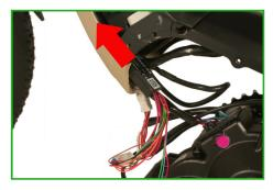
**16.** Fold the motor up again, making sure that no cables were squeezed. Reattach the motor using the previously released screws.
