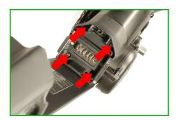
Loosen and remove the fixing screw of the right (chain side) pedal crank with a suitable allen key.
