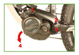
Loosen the 8-pin and white 3-pin connector on the motor. If you can not find the connectors directly, please follow the cables in the frame. The connectors are secured with a snap-in lug. Press it gently. (E.g., with a narrow slotted screwdriver)
