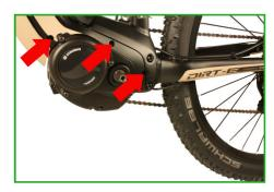
12. Loosen and remove two motor screws (1 + 2) with a suitable Allen key. <u>Attention:</u> The screws can be of different lengths! Remember this for assembling! Then loosen the third screw (3) and use it as a hinge to fold down the engine.
