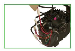
**15.** Stow all in the frame tube, the bikespeed-RS, the connectors and the cables.
