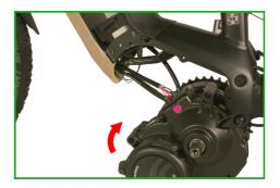
**17.** Install the engine, the covers, the chainring, the pedal cranks, the battery holder again in reverse order.
