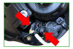
5. Remove the cable binder and move the original cables you just removed to the gap between motor and frame. Prepare the furnished cable binder for fastening the bikespeed-RS.
