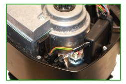
7. Connect the two removed connectors of the original cables with the white sockets on the bikespeed-RS. The plugs are coded and can only be plugged in the correct direction. Please do not use force!
