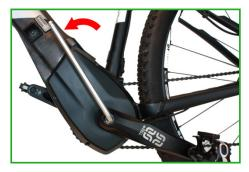
**3.** Remove the five screws of the gravel deflector and then remove it. Use a Torx T20 for untightening the screws.
