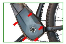
**4.** Pull the two plugs from the marked connectors and replace them with the two plug-connectors on the bikespeed-RS.
