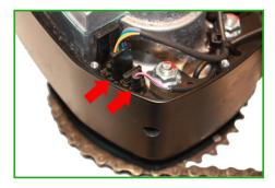
Mind the correct coding! The plugs can only be connected in one direction in the correct socket, do not use force!
