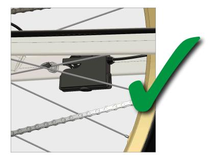
If the motor support stops while driving or an error message is displayed, calibrate the badassBox to a lower peak velocity.
