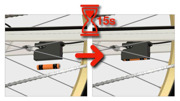
5. If the procedure is followed correctly, the badassBox is immediately in calibration mode after the battery has been inserted. The tacho of your e-bike should indicate a constant speed (even if the rear wheel does not rotate) - this is the currently set peak velocity of your badassBox, e.g.:
