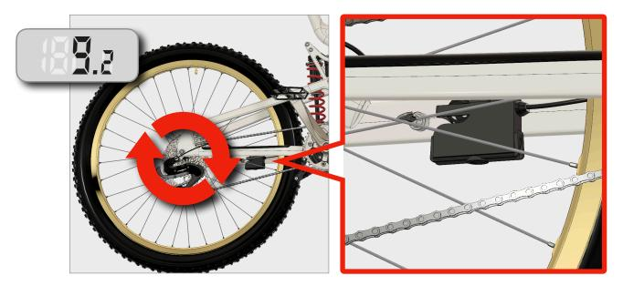
2. Now remove the badassBox from your e-bike, remove the cover and take out the battery:
