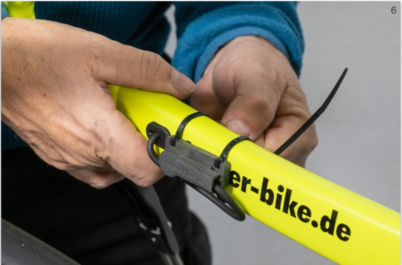
6. Attach the adapter to the frame of your bike with the supplied cable ties.
