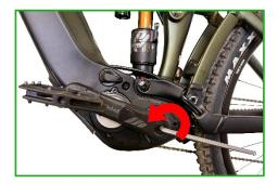
4. Loosen the four screws of the lower gravel deflector with a size 2.5 Allen key and remove it. Note: Different screws are used at the front and rear. Please note the position for later correct mounting.
