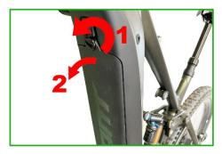
2. Loosen the battery mounting screw with a Torx T25 or your battery key. Note: This is an endless screw that cannot be removed.
