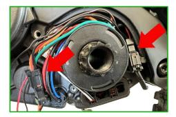
8. Replace the side cover. Guide the two remaining connectors of the bikespeed-RS out of the opening at the bottom right and guide the cable to the bikespeed-RS out of the cover on the left. (See arrow) Then fasten the cover again with the three screws. Make sure that you do not squeeze cables!
