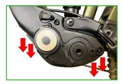
5. Disconnect the two connectors for the display (6-pin, labeled "Info") and the speed sensor (3-pin, labeled "SS"). The connectors are held in place with a latching tab. You simply release this with a slight pressure with your fingernail or a narrow screwdriver.
