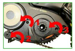
7. Connect the two connectors disconnected in step 5 to the corresponding counterparts on your bikespeed-RS and place the connectors at the locations marked with arrows:
