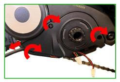
**9.** Connect the two connectors of the bikespeed-RS to the slots on the motor where you disconnected the original connectors in step 5.
