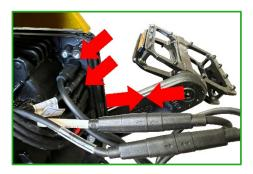
**4.** Store the tuning and cables inside the frame and reattach the cover.
