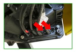
Connect the disconnected connectors to their corresponding counterparts on the bikespeed-RS. Then, connect the other two plugs on the bikespeed-RS to the available slots on the motor.
