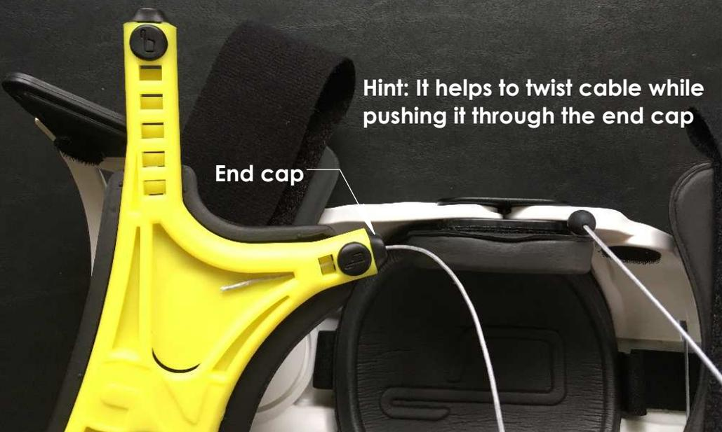
Step 30 - Push cable and cable housing through tendon back plate as shown
