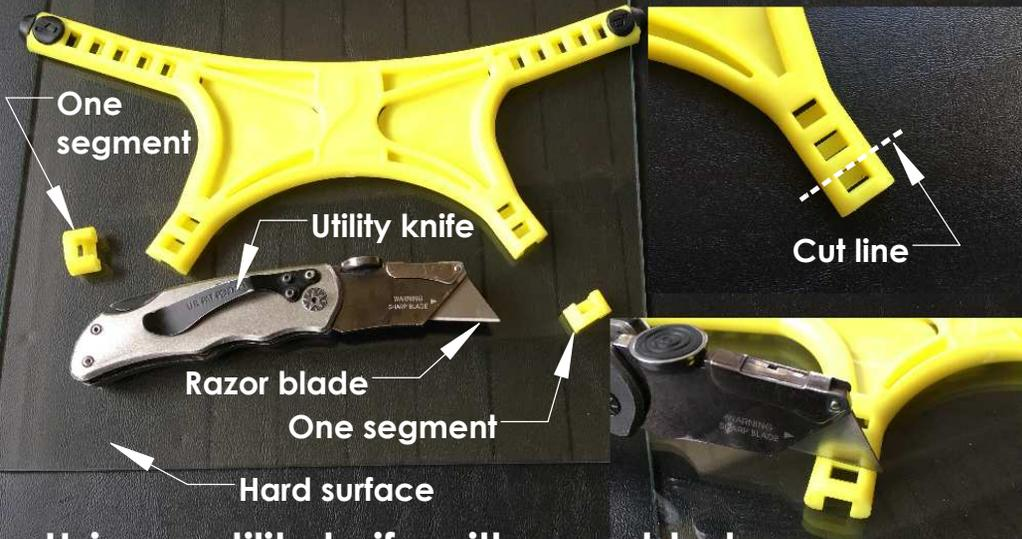
**Using a utility knife with razor blade cut against a hard surface as shown**
