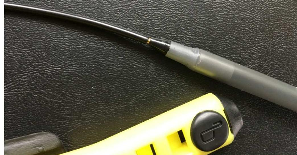
Step 28 - Push cable through tendon back plate as shown
