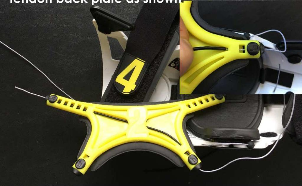
**Step 35 - Push cable through cable housing as shown**
