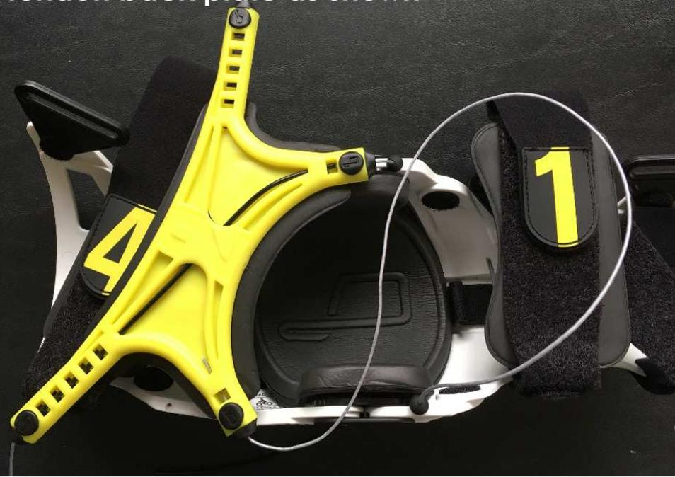
**Step 33 - Push cable housing through lower leg, and pull cable and housing back through tendon back plate as shown**
