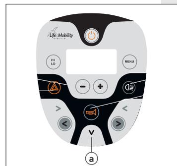
By default the speedometer is set to 4 blocks, which is 40% of the total power. The maximum speed is 7,5 mph (12 km/h). Your supplier can adjust the speed setting.
