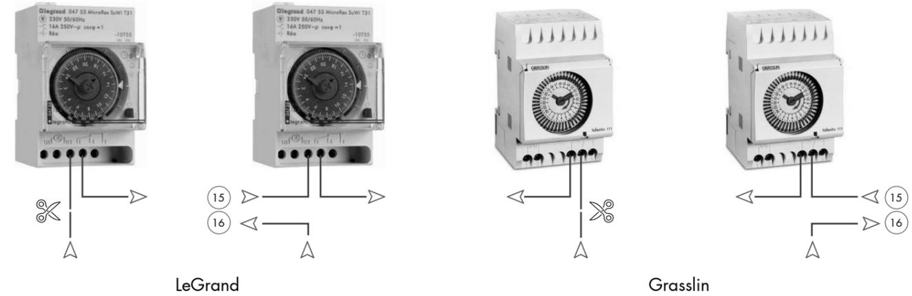
The two ends should be connected to terminals 15 & 16 on the terminal strip in the electrical compartment of the OptiClimate.
