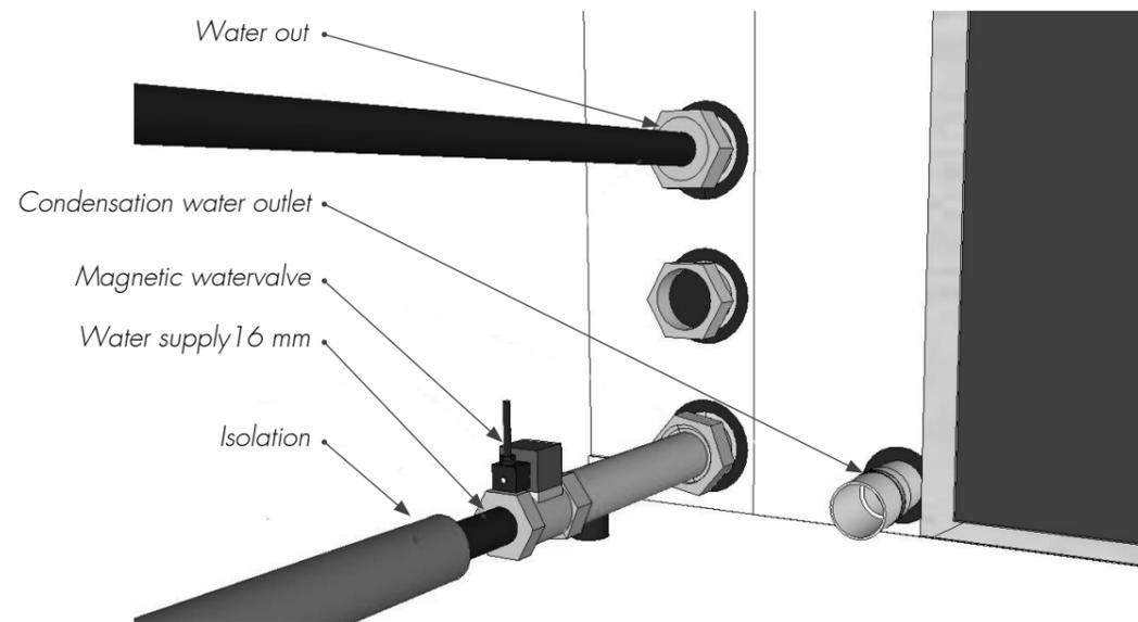
Solenoid valve in the supply pipe of the water
