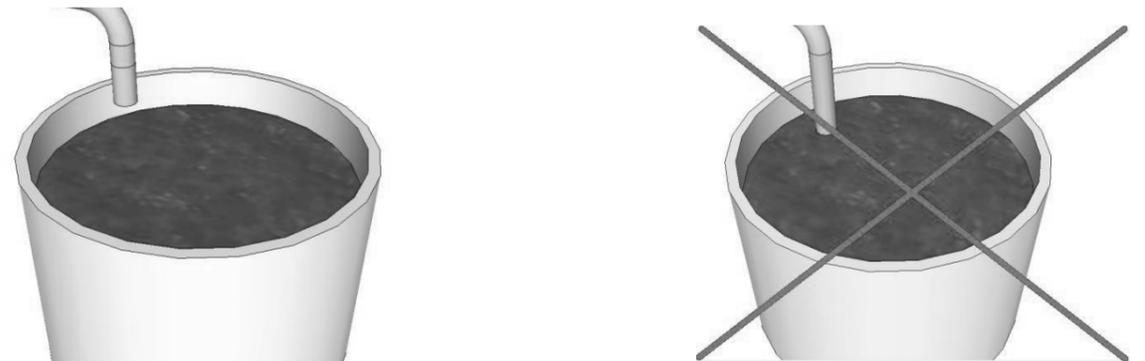
If the unit is installed at the same level or lower than the drain or sewer, a condensation lift pump can collect the water. This small lift pump pumps the water through a hose of 9mm to a height of 4 metres into the drain. Stronger pumps are also available.
