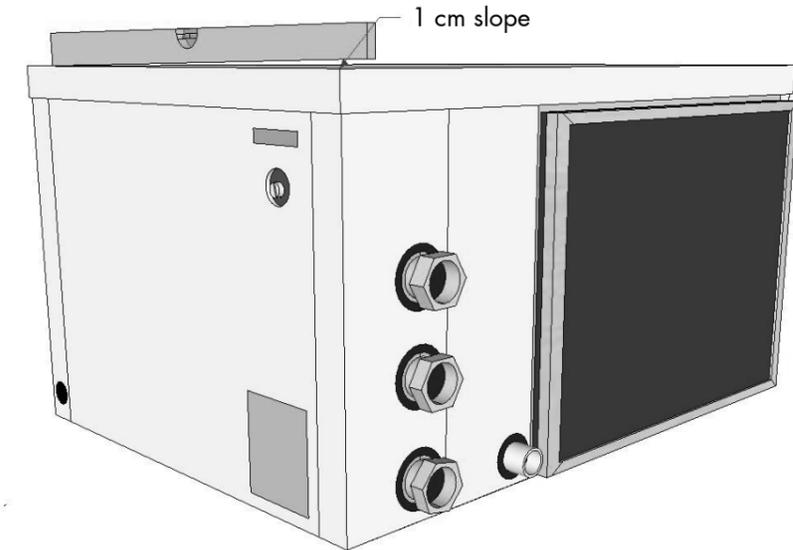
The unit should be mounted in such a way that the side of the condensation drain is at least 1 cm lower than the other side (slope) to ensure that the condensate drains properly. In practice, the 1 cm elevations at all corners – except the corner of the electrical compartment – are exactly right for a correct fall. Using a spirit level is recommended.
