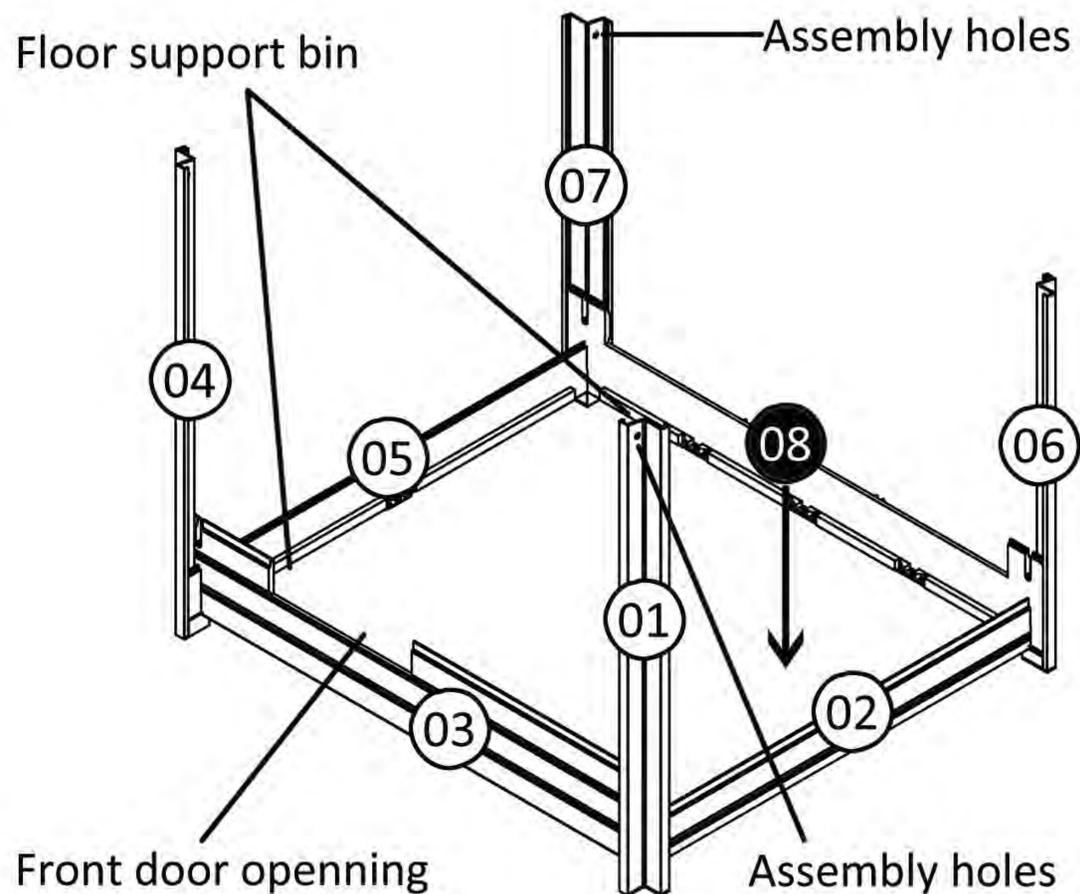
So far you have setup the wall base panels, (02) , (03) , (05) & (08) ; and the 4 column posts. Step back and stand facing the front door open. Do a quick check:
