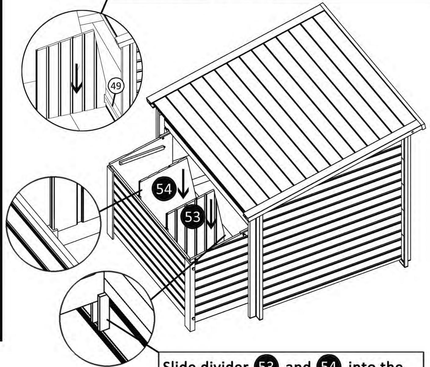
Slide divider (53) and (54) into the "u" shaped guides in the wall panels.
