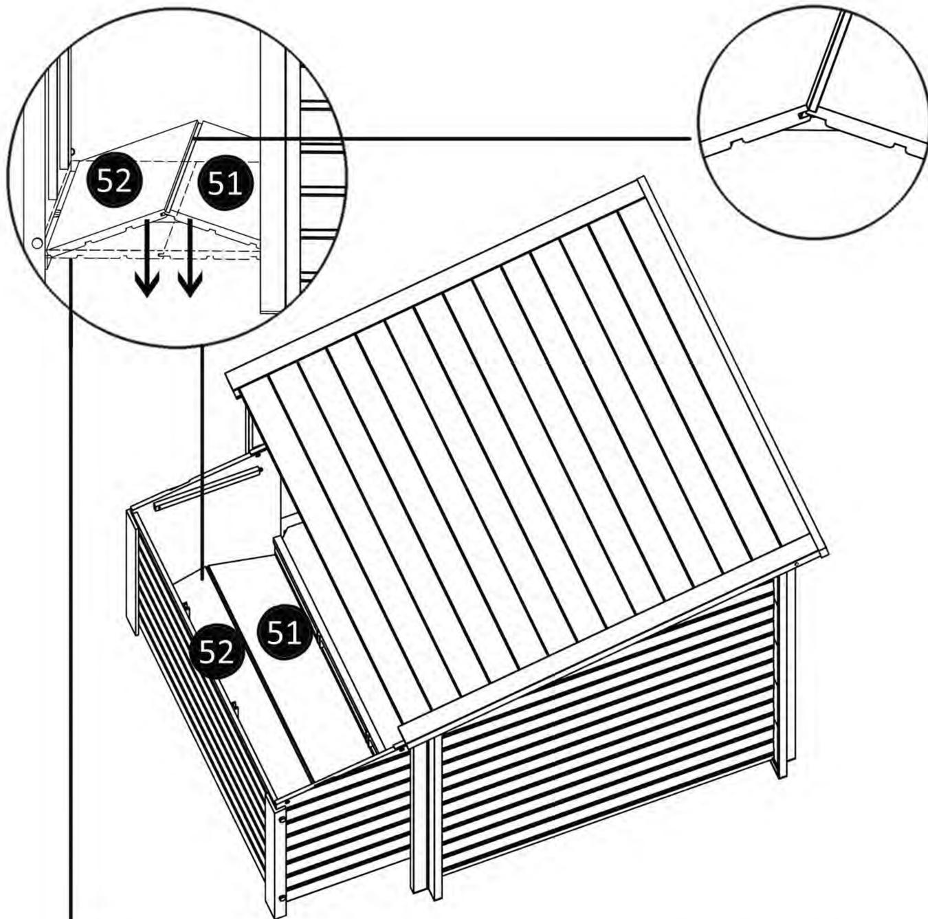
Slip the tongue of (51) into the groove of (52) and hold at an angle as shown. Position in the space as shown and push down to seat.
