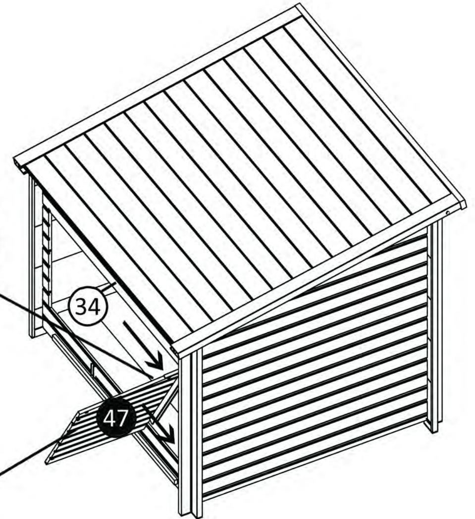
Tilt (47) as shown. Align the top of (47) with the notch in (34). Push to lower part of (47) sideways until vertical.
