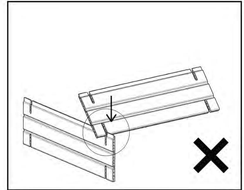
When installing wall panels, make sure the two connecting panels are at a 90 degree angle vertical to the ground, and 90 degree perpendicular to each other. Tilting in any way might cause damage to the groove.
