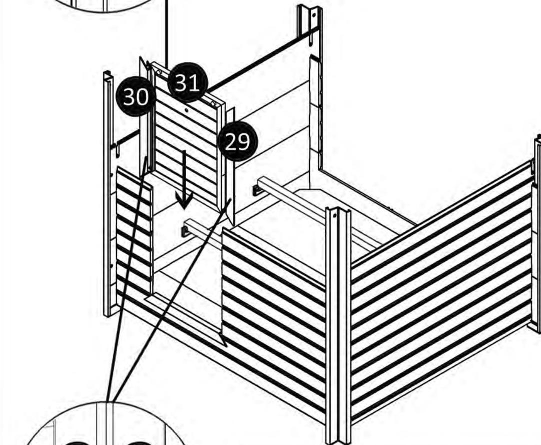
Insert one end of a pin (J) into the hole in door panel (31), the other end into the hole in door frame (29). Repeat on the other side. Place the assembled unit in the door opening as shown.
