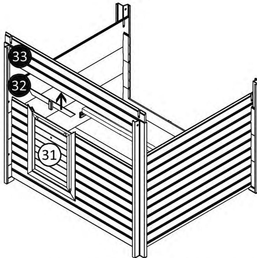
IMPORTANT: Make sure the door (31) is swung out when putting part (32) and (33) onto the structure. If you have the door swung in here, it won't be able to swing back out after part (32) is installed.
