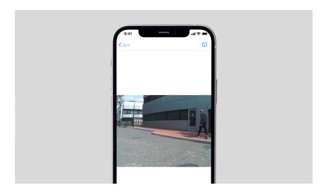
When the detector is triggered, the built-in MotionCam Outdoor camera can take 1 to 5 images with a resolution of  $320 \times 176$  and up to 3 images with a resolution of  $640 \times 352$  pixels. The detector has infrared illumination for shooting in the dark, which is activated only when an alarm is raised.
