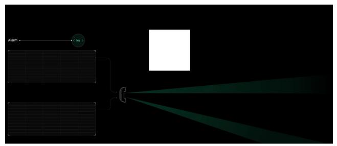
When set up and installed correctly, MotionCam Outdoor ignores animals up to 80 centimeters tall. The detector has two IR sensors and raises an alarm only when movement is detected by both sensors.
