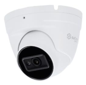
Safire Smart Range I1 with Advanced Artificial Intelligence Turret IP Camera 1/3" Progressive Scan CMOS 4 Megapixel (2592x1520) 2.8 mm Lens 0 Lux IR Range 30 m Compression H.265+ / H.264+ WDR 3DNR Integrated microphone Audio Advanced Artificial Intelligence: human, vehicle and non-motorized vehicle detection Facial Capture Video metadata Human, vehicle and non-motorized vehicle counts WEB, CMS, Smartphone and NVR interface **ONVIF** Compatible PoE (IEEE802.3af) Weatherproof IP67
