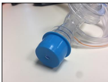
A pierced cap used on the transducer
