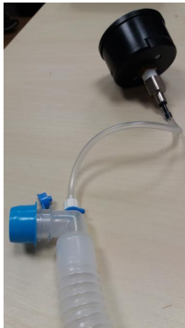
Manometer attached for VV test
