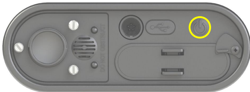
Back panel indicating the Power On/Off button
