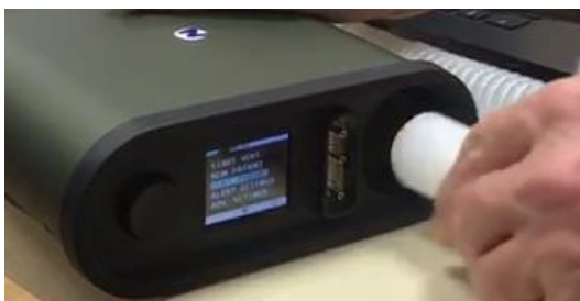
Insert ventilator tube into ventilator gas outlet
