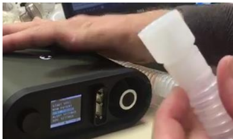
Insert ventilator tube into ventilator gas outlet
