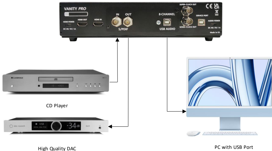
Typical signal connections of the Vanity PRO with the USB Output Module
