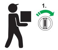
1. By turning the lock clockwise, the delivery person can open the preset lock without a key.
