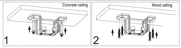
Please drill 8mm hole on the ceiling, and insert the bolt. Align bracket with the hole, then tightten with nut.
