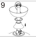
Loosen two set screws on the downrod support and then place the downrod into the downrod support. Align the Clevis Pin holes in the Downrod with the holes in the Downrod support. Be sure to push the straight leg of the Hairpin Clip through the hole near the end of the Clevis Pin until the curved portion of the Hairpin snaps around the Clevis Pin. Finally, re-tighten the two set screws.
