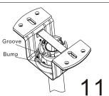
Carefully lift the fan, and set the downrod/ hanger ball assembly on the hanger bracket attached to the ceiling. Be sure the groove in the ball iss properly aligned with the tab on the hanger bracket.
