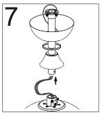
Remove and save the clevis pin and hairpin of the downrod. Put the downrod through the canopy and coupling cover. Thread the electrical wires and the earth wire through the downrod.
