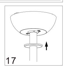
Mount the canopy by tighten the two screws
