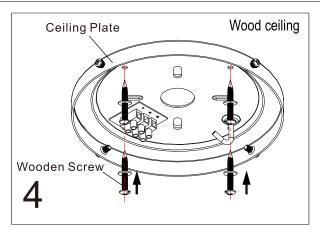
Please drill 8mm hole on the ceiling, and insert the bolt. Align bracket with the hole, then tightten with nut.
