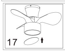
1, put the diffuser into the plate, then rotate it clockwise ockwise (like picture 14 showed)
