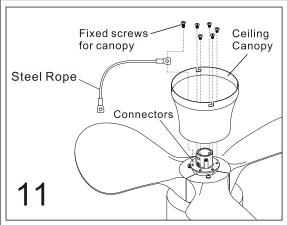
Fixed the canopy and steel cable to the connector by the screws, like the right picture showed
