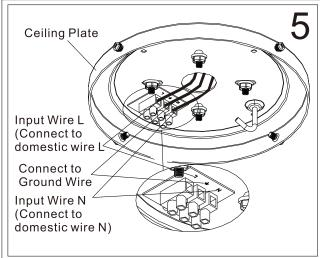
Connect the domestic live wire to the terminal L, null wire to the terminal N, earth wire to the terminal earth position
