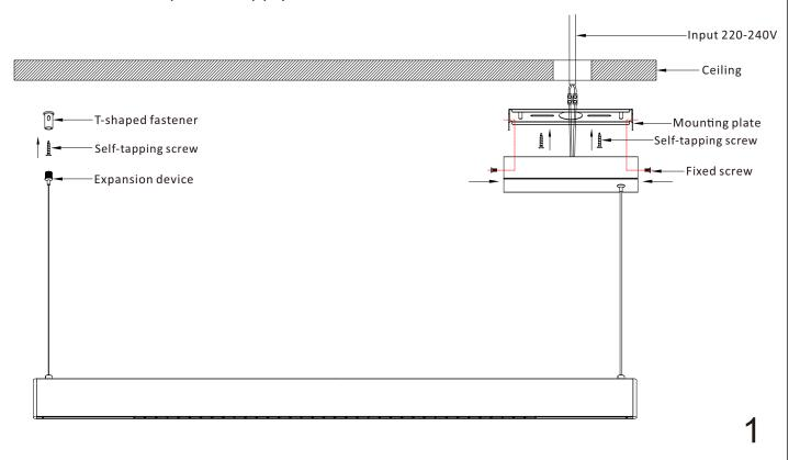
Fix the hanging plate and the ceiling box with the fixing screw, push the wire rope into the expansion device and pass through the hole on the side of the T-shaped fastener, lock the safety piece, adjust the wire and wire rope to the appropriate height and then power on.
