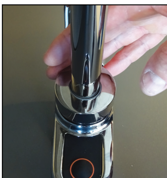
Step 5 Place the nut over the new spout.
