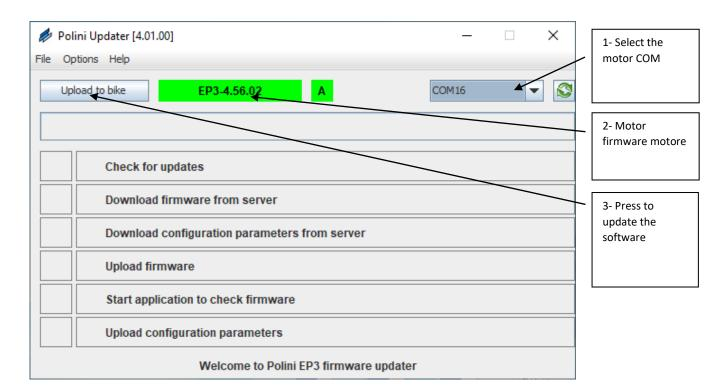
• The program will shows the version of the firmware already installed on the motor, press the key "Upload to bike "at the top left. If a new version of the firmware is available on line, it will update automatically; otherwise it will be confirmed that on the motor the last version available has been already installed. Once the update has been completed, disconnect the USB cable, switch the bike OFF and then switch it ON.
