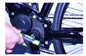
Using a Torx 20 key remove the plastic cover
