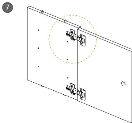
Mount the doors onto the side panels of the cabinet.
