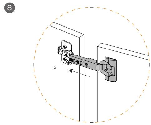
Slide the hinge over the metal plate.
