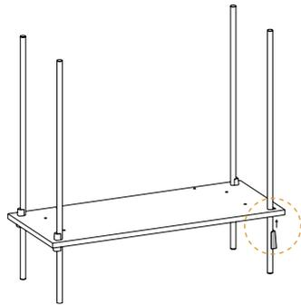
Start by placing the bottom shelf at a desired height, fasten it with the wedges. Use a water level and a hammer to make sure it is leveled and secured.
