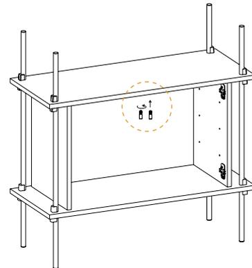
Insert the door stoppers by screwing them into the holes of the top shelf.
