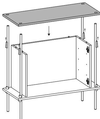
Slide down the top shelf until it sits on the dowels of the side panels. Fasten it with the wedges. Use a hammer to make sure it is secured.
