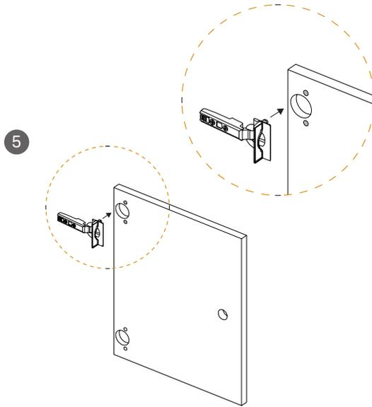
Place the hinges in the large holes of the doors.
