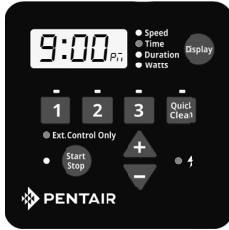
Figure 7: Activating External Control Only
