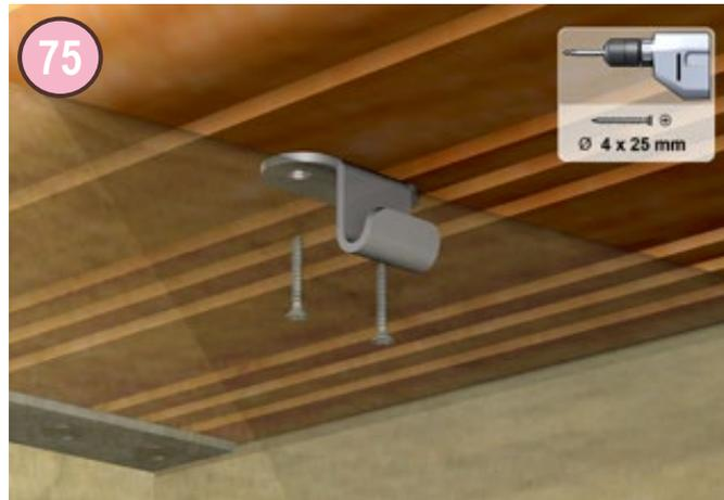
The wooden ladder is fitted with two lever latches that lock it into position. The lever sections are fitted to the ladder supports and the hooks are mounted under the coping (these parts are enclosed in bag K). Observe how these 2 parts interact together to understand how the mechanism works and establish the travel necessary for the ladder to be locked correctly into position.
