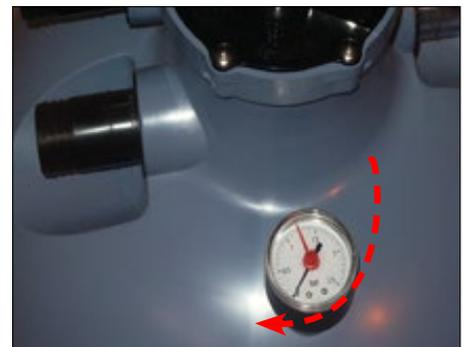
Working from underneath the cover, tighten the bronze nut by hand, then moderately using a 22 tube wrench. Take care not to damage the o-ring.
