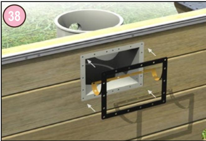
Before fitting the liner, glue one of the 2 rectangular self-adhesive gaskets (pool fitting skin pack) around the mouth of the skimmer or filtration unit.
