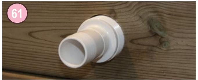
Wrap Teflon (not provided) 3 times around the threading of the hose tail before screwing it onto the body of the skimmer. Fit the pump suction line onto the skimmer hose tail and fix it in position using a circlips.
