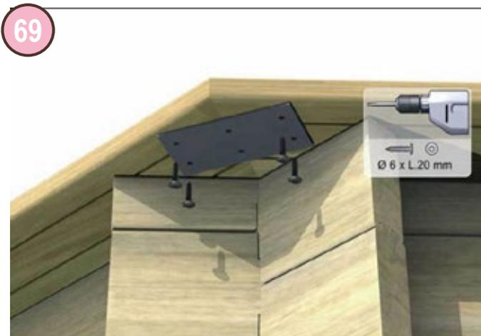
All that remains is to attach the 8 coping corner connecting brackets (bag 27511671) as shown above, taking care to position the brackets correctly..
