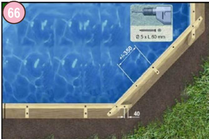
Attach the 7 coping planks of the same length. Be careful to drive the screws into the centre of the wooden walls to avoid damaging them. (screws from bag T or Q)
