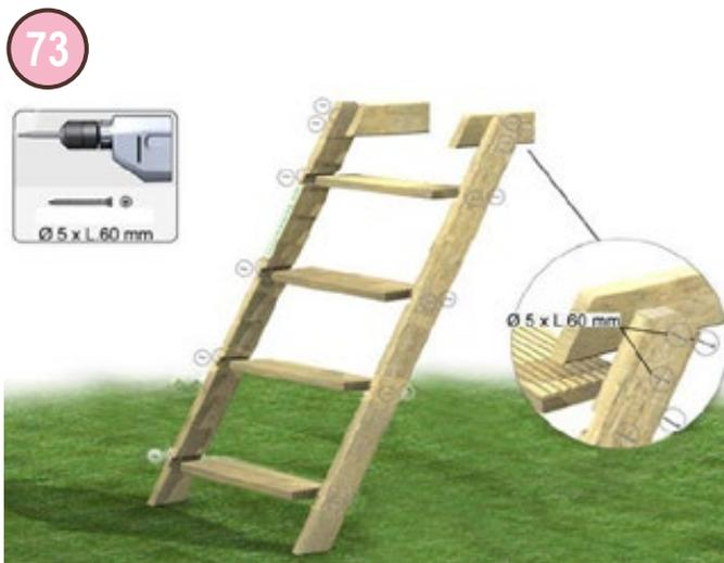
The stringers and the treads for the wooden steps are in the Wood kit. Assemble the wooden steps using the SS screws (bag K). For cleaner, more efficient assembly, we recommend that you pre-drill the various elements (4 mm drill bit) and mill the holes to avoid splitting the wood and raising splinters.
